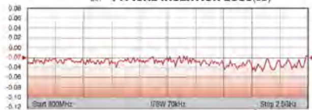
S21 TYPICAL INSERTION LOSS (dB)
