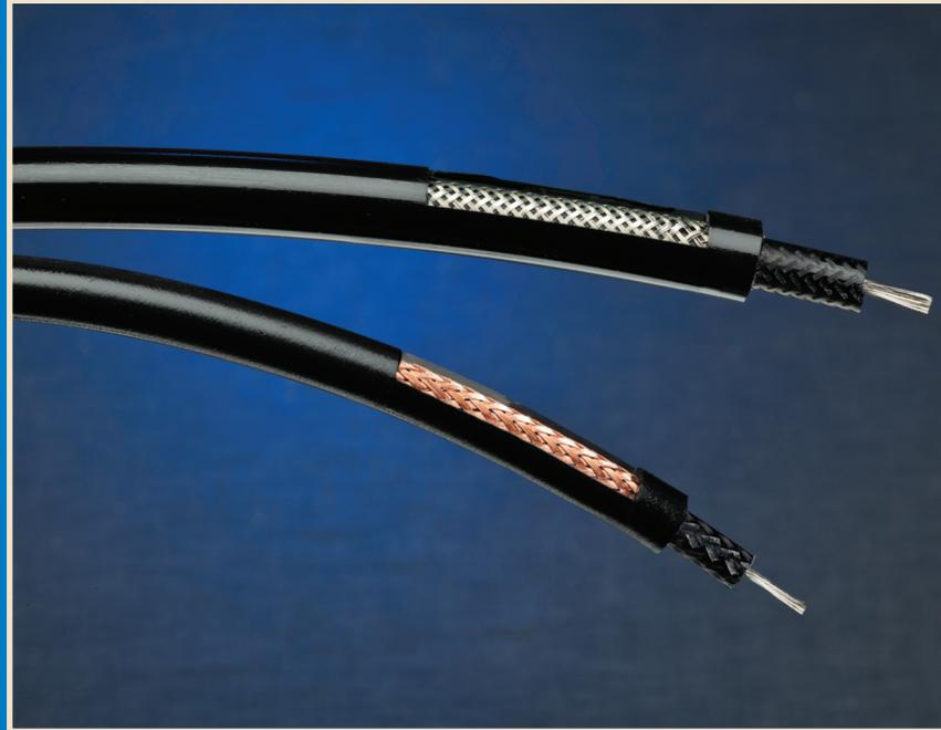
T-LNC™ 50 and 75 Ohm low noise coaxial cables employ a combination of semi-conducting and insulating dielectric layers to achieve optimum low noise performance. T-LNC™ cables are the perfect cable solutions for noise-sensitive applications such as vibration and wear monitoring and detection as well as low voltage signaling in high vibration environments.
