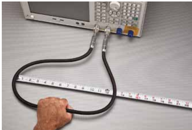
Flex Test (one full cycle)
