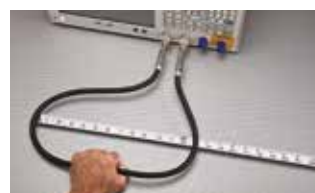
Flex Test (one full cycle)
