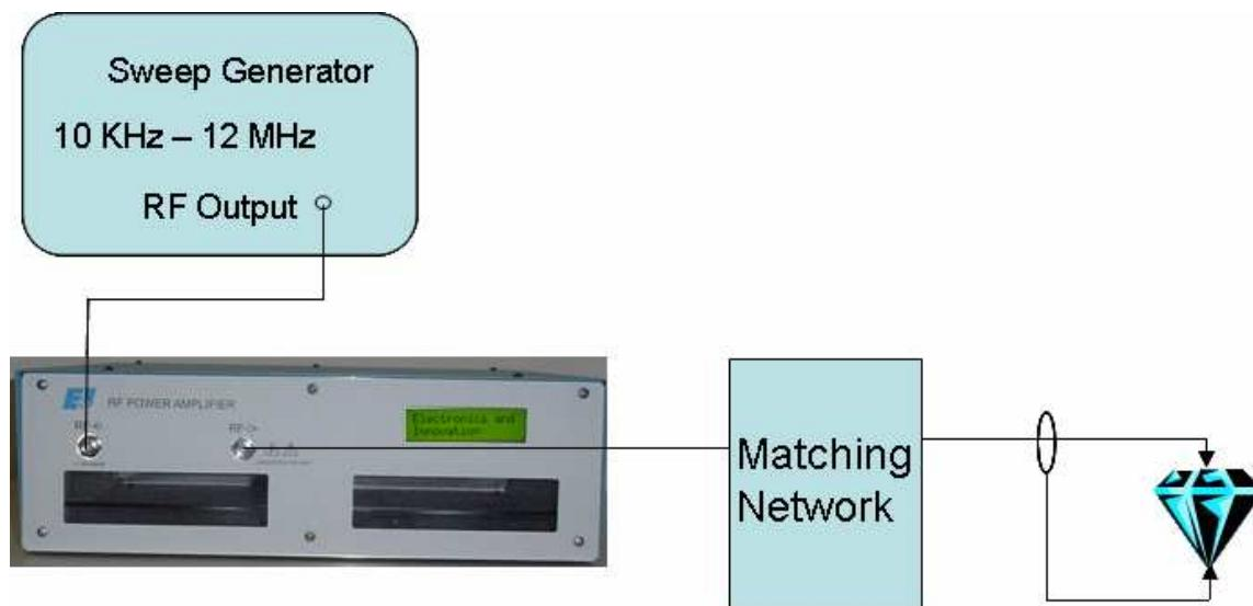
Refer to the chart labeled "Complex Impedance of a NaCl Crystal" At a frequency of 1 MHz a series inductor can be selected to have an inductive reactance ( $X_L$ ) of +j 7557
