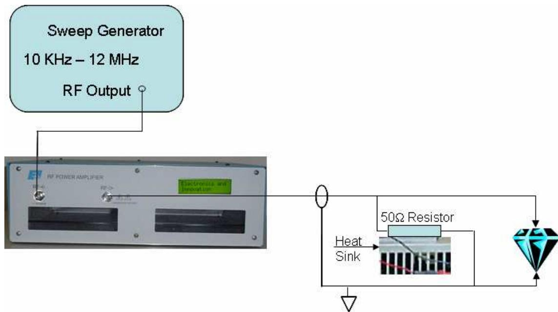
The complex impedance of the same NaCl crystal and a 50 Ohm resistor was measured and is shown below.
