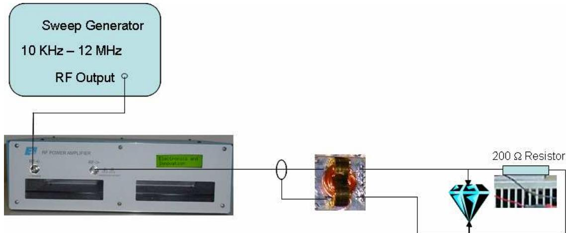
A broadband auto transformer can be employed to step the voltage up by a factor of 2, 3, or 4 depending on the transformer topology that is selected. The same salt crystal was terminated with a low inductance 200 Ohm resistor and the complex impedance was tabulated.
